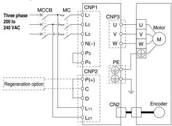
\* For single phase 200 to 240 VAC, power supply should be connected to L₁ and L₃ terminals, with nothing connected to L₂. Please note that the wiring locations differ from the LECS□.
