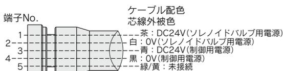
結線図 (PROFIBUS DP, EtherCAT, PROFINET, Ethernet POWERLINK, PROFI-safe, Safety over EtherCAT®)
