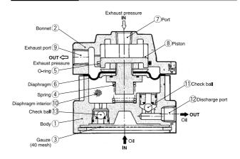
When the exhaust pressure from the switching valve enters into port  $\bigcirc$ , the piston  $\bigcirc$  and diaphragm  $\bigcirc$  compress and displace spring  $\bigcirc$ , the exhaust pressure is released into the atmosphere from exhaust port  $\bigcirc$ , and at the same time the diaphragm is returned to its original condition by the recovery power of the spring.
