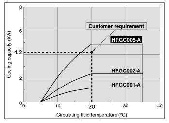
The point plotted in the graph is the requirement from your customer. Select the Thermo-cooler models exceeding this point. In this case, select the **HRGC005-A**.
