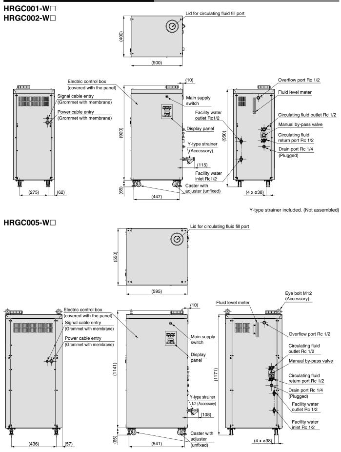
Y-type strainer and eye bolts included. (Not assembled)
