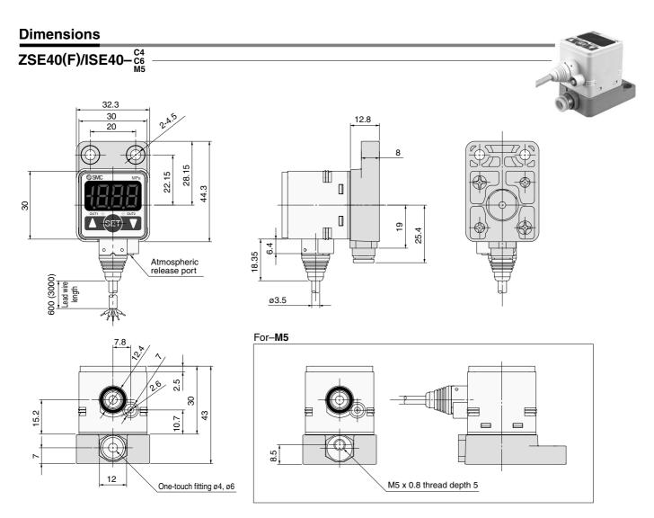
\* For splash proof use (IP65), insert an air tube into the atmospheric release port. (Refer to "Precautions" for details.)
