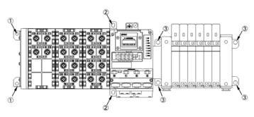
All manifolds are mounted using 8 screws (except VQC4000 which uses 7 screws).
