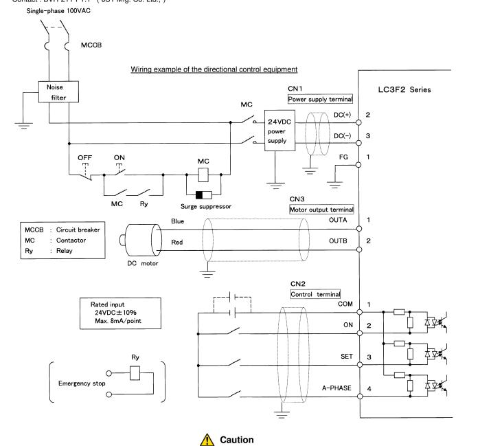
Directional control equipment does not have an emergency stop or power on/off switch. Provide an emergency stop, circuit breaker (protection) for the total system, referring to the wiring example above.
