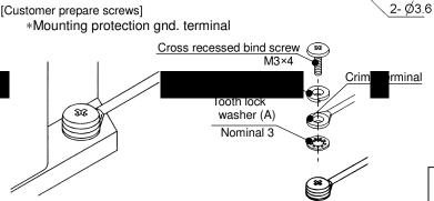
Customer prepares crimp terminals and ground cable.
