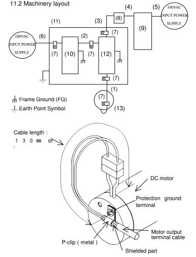
Fig.1 How to ground the DC motor (Type3)
