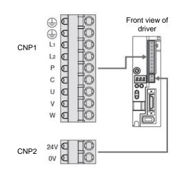
Main circuit power supply connector (CNP1)
