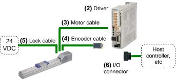
(1) Electric Actuator – Slider type
