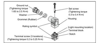
Figure 5. DIN exploded view for SF4. VQZ and VK pilot valves
