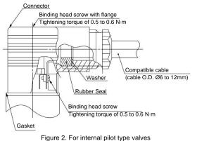
If using cable with outer diameter of Ø9-12 mm, remove inner part of rubber seal before use.
