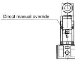
Figure 2. VFR3000 Direct manual override location
