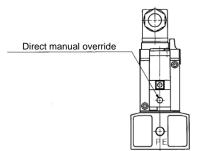
Figure 3. VFR4000 Direct manual override location
