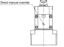
Figure 5. VFR6000 Direct manual override location
