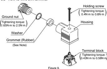
Applicable cable - O.D. Ø6 mm to Ø12 mm. Inside bore of grommet will need to be trimmed if cable O.D. is >09 mm.
